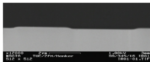
Cross sections of the grooves of the standards with a depth of 0.09 \mu\text{m} : rounded sidewalls
