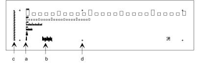
For the calibration of profiling instruments in view of the length of a profile (scan length) a line scale standard is available that contains periodically arranged grooves. The lateral distances inside the periodic profile are defined very precisely by sharp edges of grooves:
