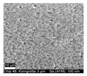
The rough surface is formed by a lapping process. The resulting roughness mainly depends on the size of the used grains. The rolling grains break off particles from the surface and produce deepenings which are randomly distributed. Consequently the roughness is uniform and independent on the direction at the surface and therefore suitable as an isotropical areal roughness standard.
